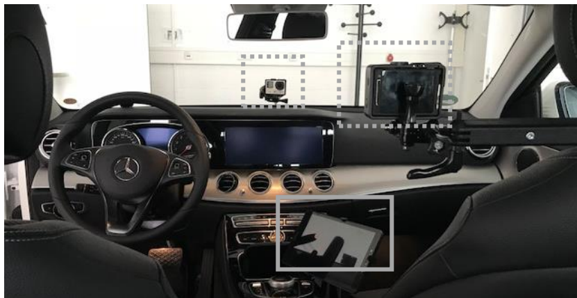
Figure 3.3.1. Position of the tablet running the emotion tracking application (solid line) and the cameras (dotted line).
