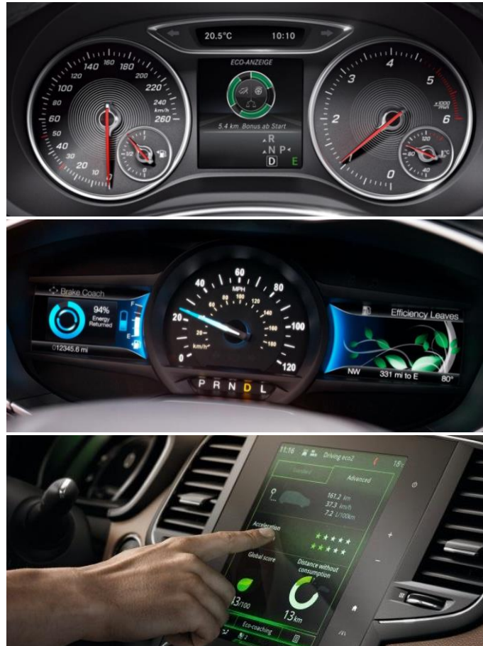
Figure 2.3.2. In-car interfaces to support ecological driving developed by Mercedes-Benz (top; 2020), Ford (middle; 2016), and Renault (bottom; 2019).
