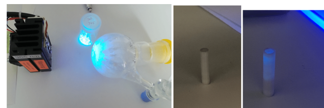
Figure S25. Left: brightly luminescent polymorph of 2b irradiated with 365 nm before solid state MAS NMR experiment. Middle: the same sample of 2b irradiated with 365 nm after solid state MAS NMR experiment. Right: the same sample of 2b irradiated with 254 nm after solid state MAS NMR experiment. The NMR measurement conditions apparently lead to a phase transition.
