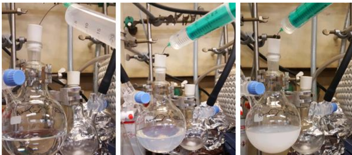
Figure 5.1.9. Images of particle formation of 3c recorded during addition of a solution of 1 to a solution of 4c in acetonitrile ( Route B ). From left (1) to right (3): (1) before addition, (2) after addition of 10 mL of a total volume of 25 mL, (3) after addition of 15 mL of a total volume of 25 mL.
