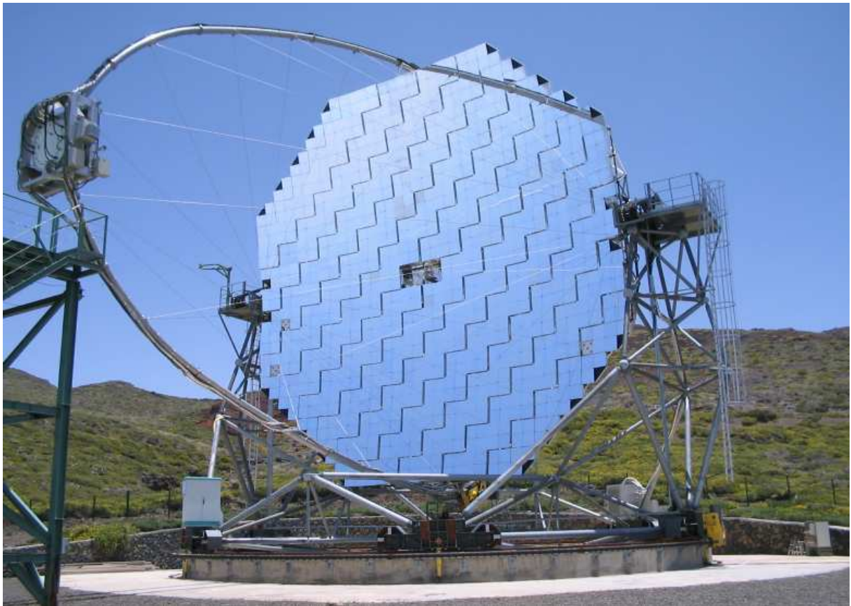
Figure 2.2.: MAGIC telescope during daytime in park position. In the center of the dish two panels are left out to provide space for the calibration box (section 2.1.5) and some CCD cameras for the active mirror control (section 2.1.3) and the calibration and monitoring of the pointing (section 2.1.2).
