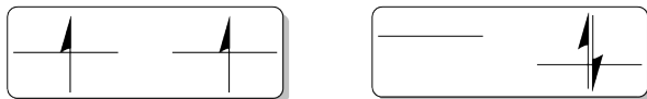
Figure 2.1.: Orbital changes from the undistorted (left) to the JT distorted molecule (right).
