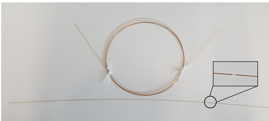
Figure 1. Fused silica capillary (BGB Analytik, 363 \mu\text{m} OD, 75 \mu\text{m} ID) employed in CE, shown wound up (top) and cut to 50 cm length (bottom). The capillaries are covered with a polyimide layer to improve flexibility and handling. The detection window (shown enlarged) was created by carefully burning away the polyimide layer at this place. Photo was taken by the author.
