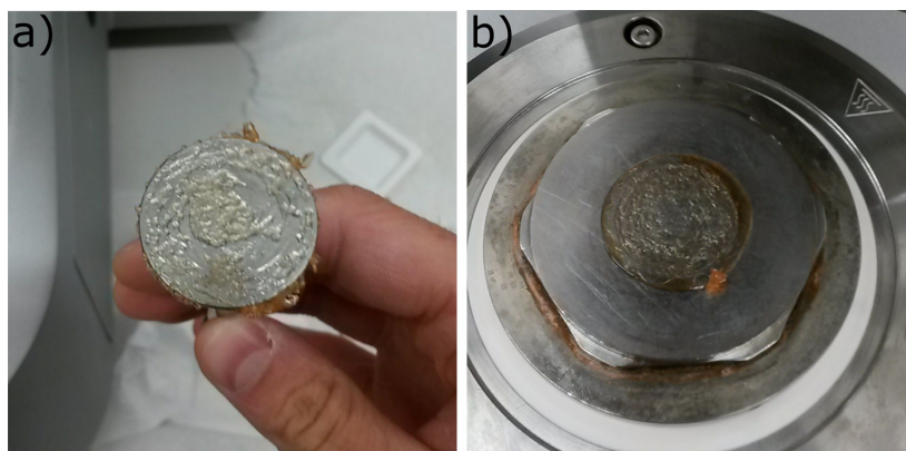
Figure 8.7: a), b) Thermally degraded DA material after a rheology measurement at ambient conditions. The material experiences a colour change from colourless to a red/brownish colour. While at the air/polymer interface the material can not be liquefied by increasing the temperature, the polymer directly under the measurement head is still liquefiable.
