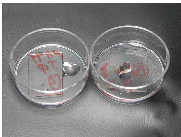
Figure 8.13: Two bulk hydrogel samples prepared from a mixture of P50 + P51 after incubation for 8 d in aqueous solution buffered to pH 11. While the sample on the left has lost its structural integrity, the sample on the right is still visibly unaffected.
