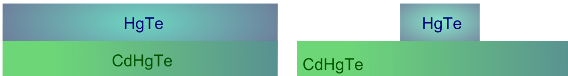
Figure 3.4: a) Schematics of the CdHgTe and HgTe layers. The HgTe layer has a nominal thickness of t = 88 nm. b) Schematics of remaining structure after dry etching, which is dubbed as “mesa”. The mesa has a height h \approx 100 nm.
