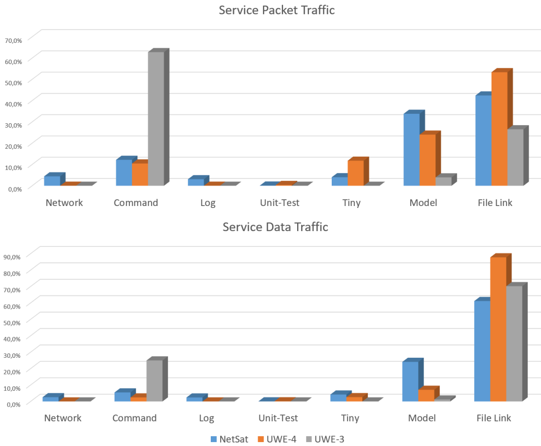
Figure 9.3: Comparison of the relative packet and data traffic of different services used in UWE-3, UWE-4 and NetSat missions. The analysis was performed using the entire recorded space-ground traffic – in total over 1.5 million packets – of the corresponding missions.
