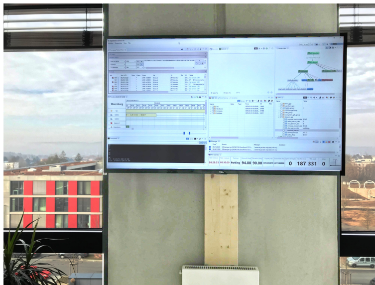
Figure 7.12: Wall-mounted monitor in all ZfT's offices as a part of the distributed mission control approach
