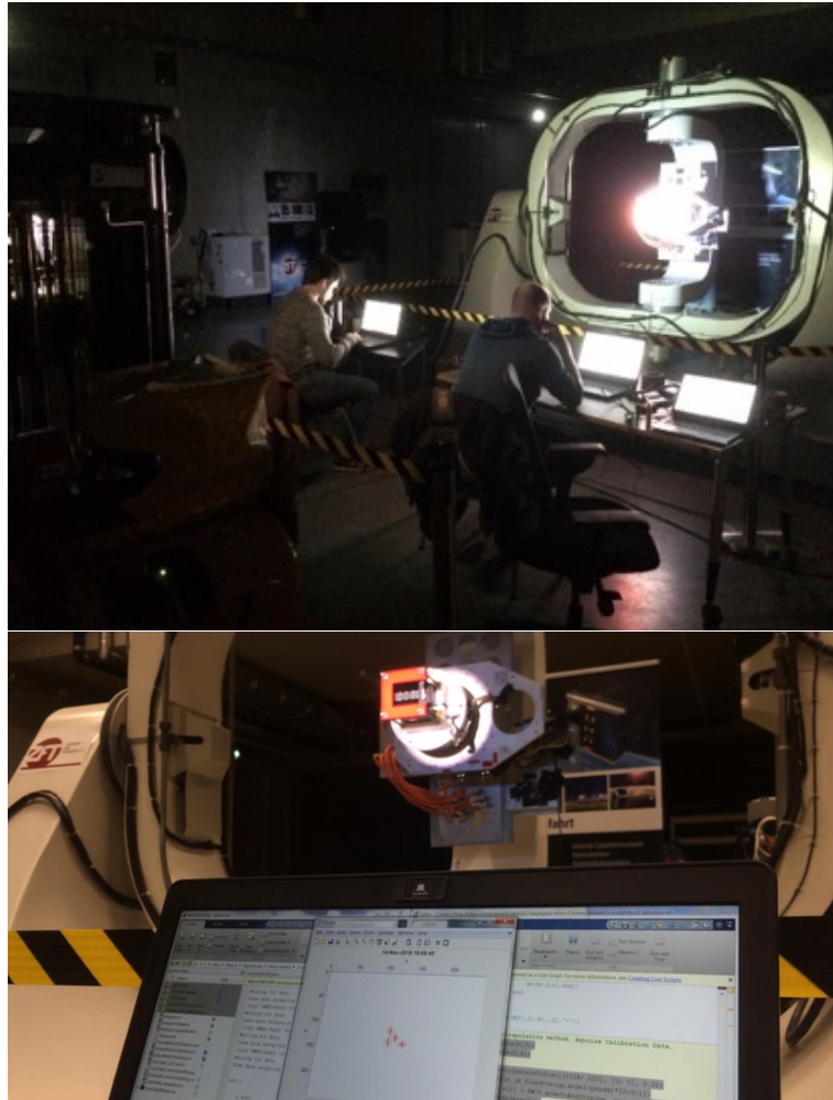
Figure 7.9: UWE team performing pre-flight sensor calibration of the UWE-4 nanosatellite
