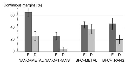
**Figure 5.** Mean percentages with standard deviation of continuous margins in enamel (E) and dentin (D) in all groups; NANO = Tetric EvoCeram; BFC = Tetric EvoCeram Bulk Fill; METAL = metal matrix band, TRANS = transparent matrix band.
