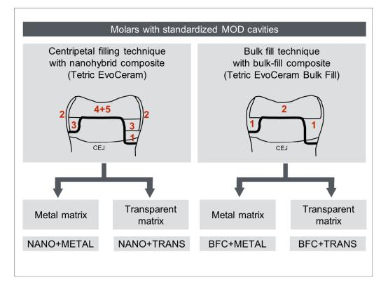
**Figure 3.** Experimental setup with the four experimental groups; red digits represent the order and number of composite increments. NANO = Tetric EvoCeram; BFC = Tetric EvoCeram Bulk Fill; METAL = metal matrix; TRANS = transparent matrix; CEJ = cementoenamel junction.
