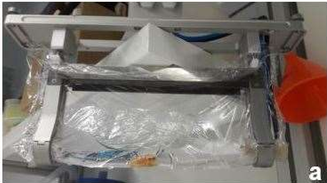
Fig. 9a. Experimental setup to create the photoacoustic images of the preliminary experiment. The tooth was held in a place in a plastic film attached to the holder and covered with water.
