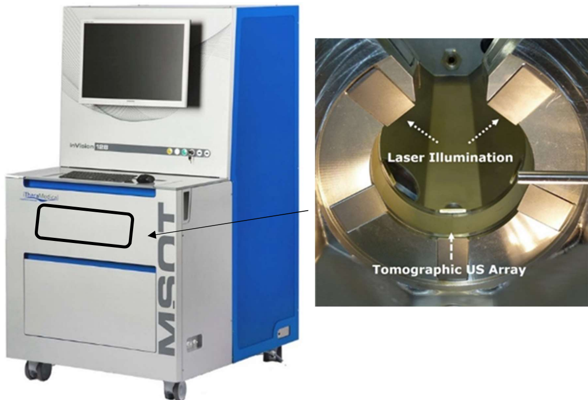
Fig. 8. MSOT inVision 128. (Left) The MSOT inVision 128 was used for the pilot study. (Right) For ultrasound detection, 128 toroidally focused ultrasound transducers organized in a concave array of 270-degree angular coverage were used. With permission from: https://www.ithera-medical.com/products/msot-invision/ .
