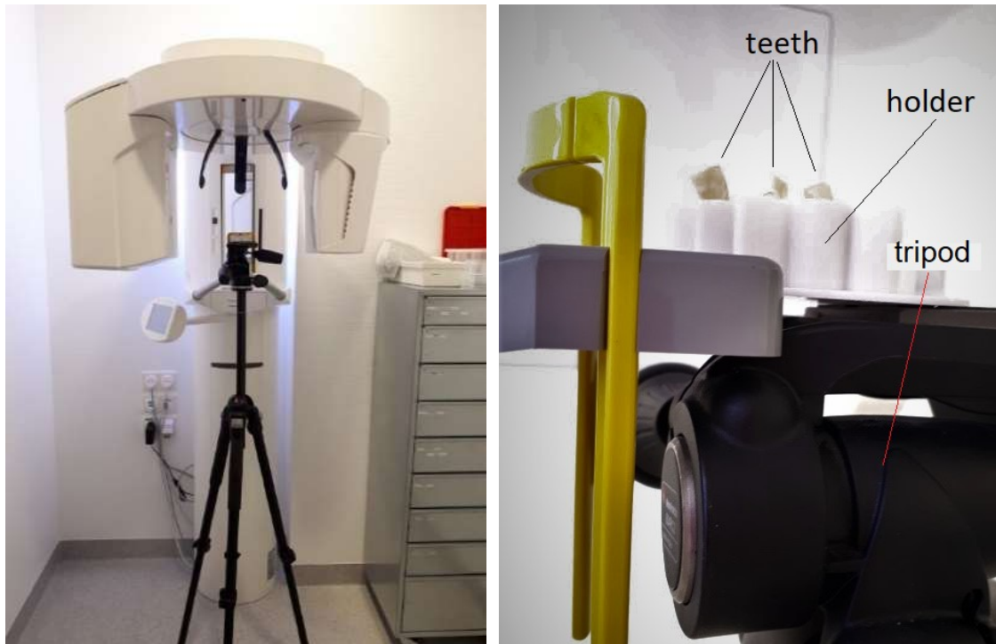
Fig. 12. Experimental setup to create CBCT images. (Left) Overview image of the CBCT device and tripod. (Right) Detailed image of the tripod with plastic holder and teeth.
