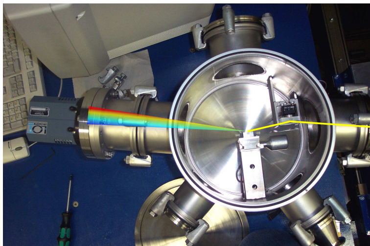
Figure 3.10: Photographic top view of the spectrometer chamber with an illustrated ray-tracing. The divergent harmonics hit the second toroidal mirror (identical in construction to the first one) which images the spectrally split XUV beams onto the X-ray CCD camera.
