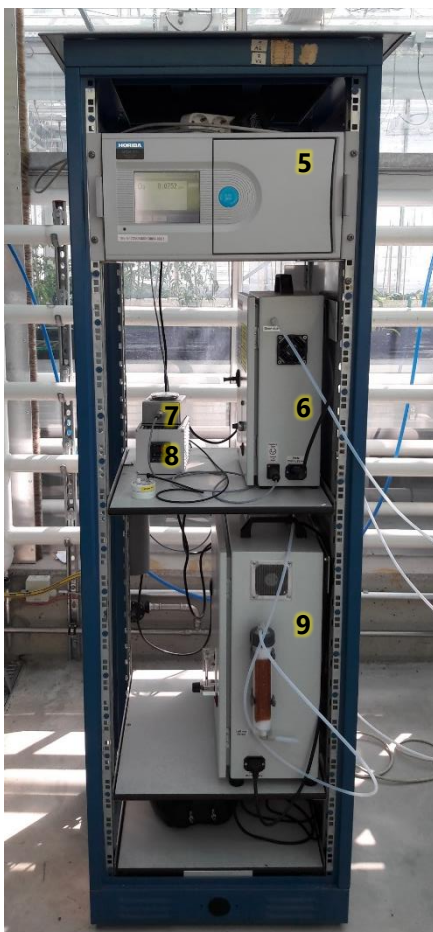
Figure I.1 – The fumigation system. A) The glass chambers. 1 – Glass chambers; 2 – Flowmeters; 3 – Activated charcoal filter; 4 – Particle filter. B) The electronic devices. 5 – Ozone analyzer; 6 – Ozone generator; 7 – Timer; 8 – Controller; 9 – Air dryer.
