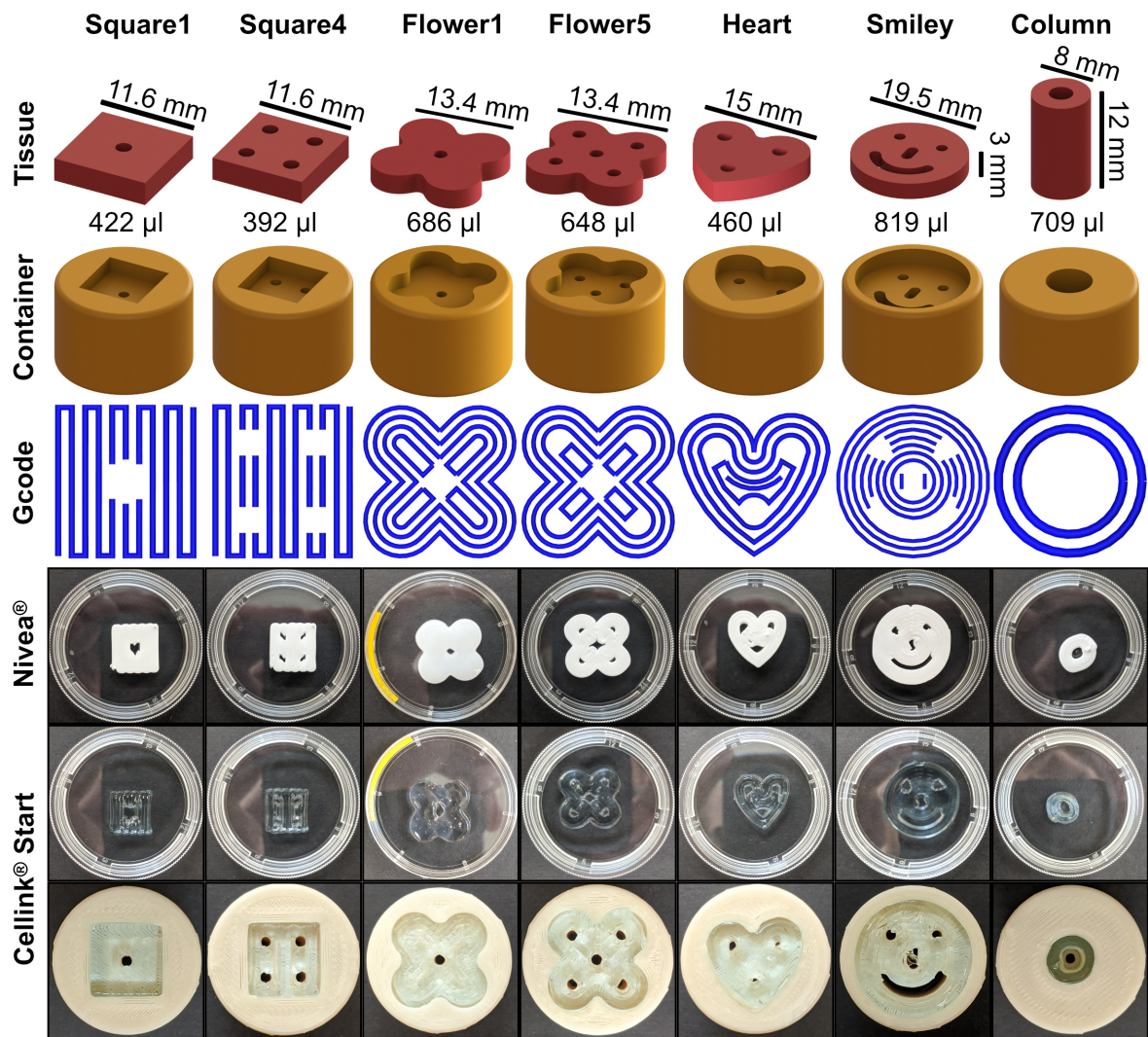
Figure 24: Proof of concept by testing different geometries from tissue design to final printing assessment. First row shows the CAD of different tissue geometries including different pore arrangements and the overall tissue volume. Second row shows the CAD of the derived tissue container. One layer of the tissue Gcode is graphically depicted in the third row. Within the fourth row first printing tests with NIVEA® lotion are depicted. The lower two rows show the bioprinting assessment using the Cellink® Start hydrogel for printing the constructs in a petri dish, as well as into the preprinted tissue container.
