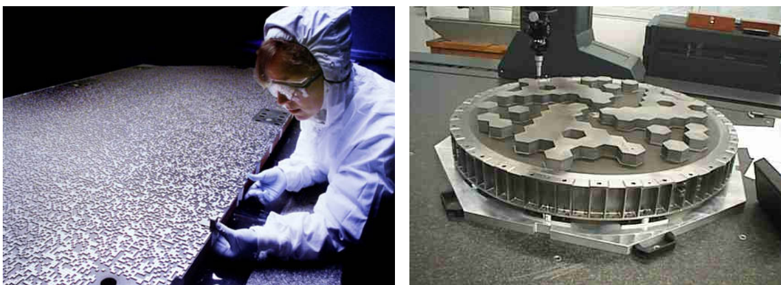
Figure 2.2.3.: Left: Coded mask aperture of the Swift BAT imager, image credit: NASA/Goddard, right: hexagonal coded mask of the INTEGRAL SPI spectrometer, image credit: INTA, Spain.
