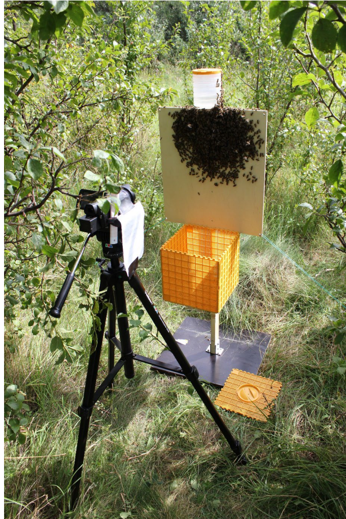
Figure 2: Swarm observation mount to assess dispersal distances of a honey bee colony.
