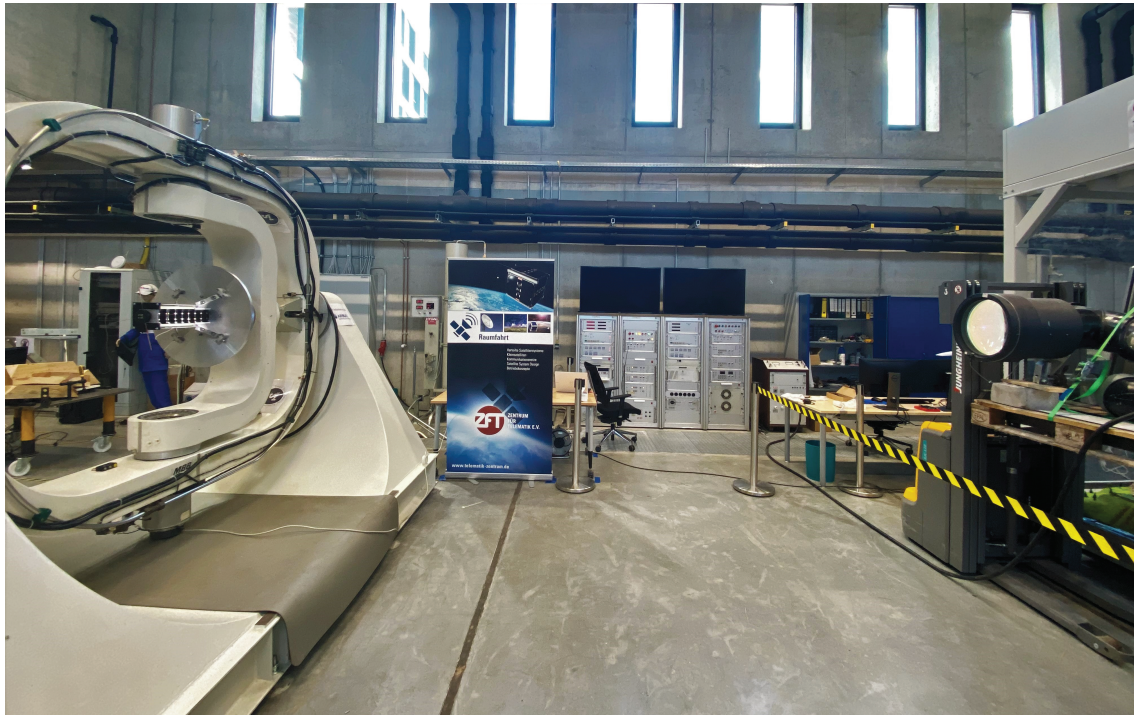
Figure 4.5: Calibration and verification setup for a sun sensor using a dynamic test facility (turn tables) and a sun simulator. The 3U CubeSat with the sun sensor is placed on the turn table on the left hand side, which can perform highly precise orientations, and is illuminated by the sun simulator on the right hand side. (Image courtesy: S4 - Smart Small Satellite Systems GmbH)
