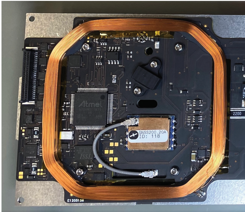
Figure 4.11: Inner side of the NetSat 3U side panel holding the magnetorquer. (Image courtesy of the author.)
