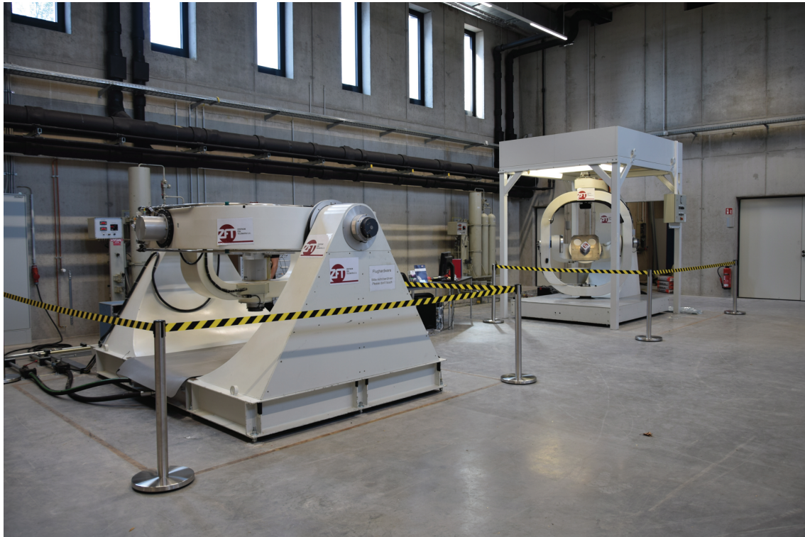
Figure 4.2: Dynamic test facilities (turn tables) at S4 - Smart Small Satellite Systems GmbH, Würzburg providing high accuracy pointing and rotation to test attitude sensors. (Image courtesy: S4 - Smart Small Satellite Systems GmbH)
