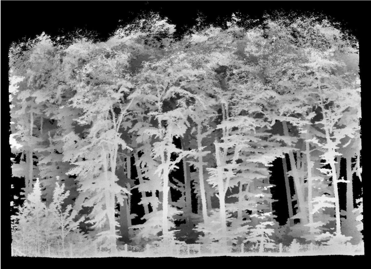
Fig. 3: Exemplary point cloud of a forest stand obtained from mobile laser scanning through a 10 min walk-through with the hand-held ZEB Horizon scanner.
