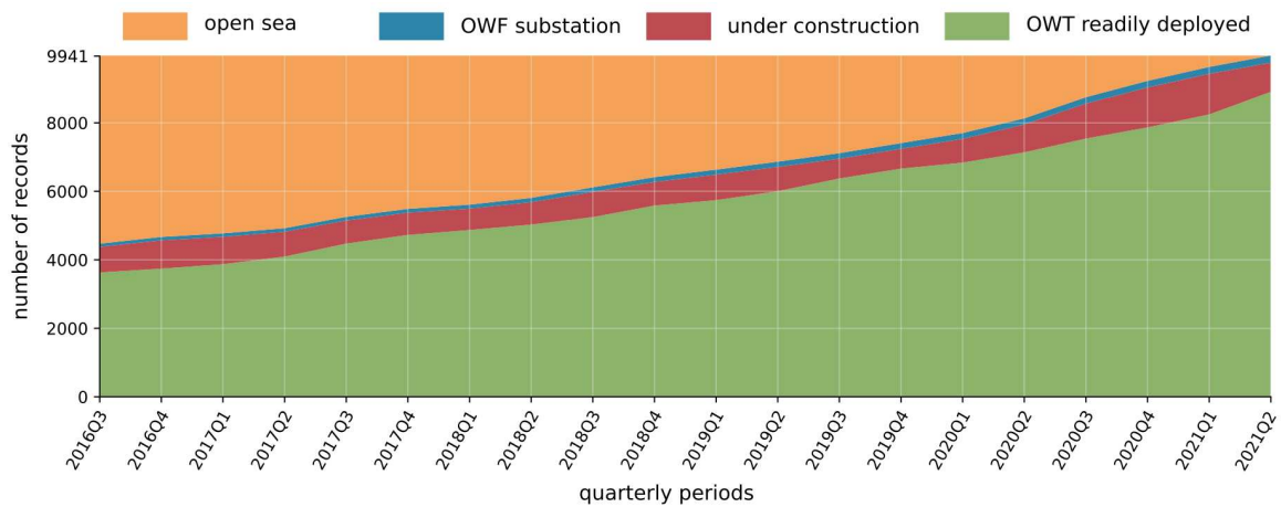
Figure 5.9: Temporal development of the 9,941 globally detected offshore wind energy infrastructure locations (offshore wind farm (OWF), offshore wind turbine (OWT)) from July 2016 until June 2021. Source: Hoeser et al. (2022, p. 4263).
