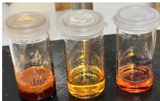
Figure 30: Photography of mixtures of different acryloyl chlorides and TEA in DCM at rt. Left to right: Commercial phenothiazine stabilized, distilled, distilled with added phenothiazine.
