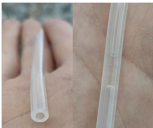
Figure 58: Photography of a casted tubular construct from 5 % HAA (8-15 kDa, 98 %) formulation in profile view of the cross section (left) and top view with meniscus after perfusion with PBS (right).
