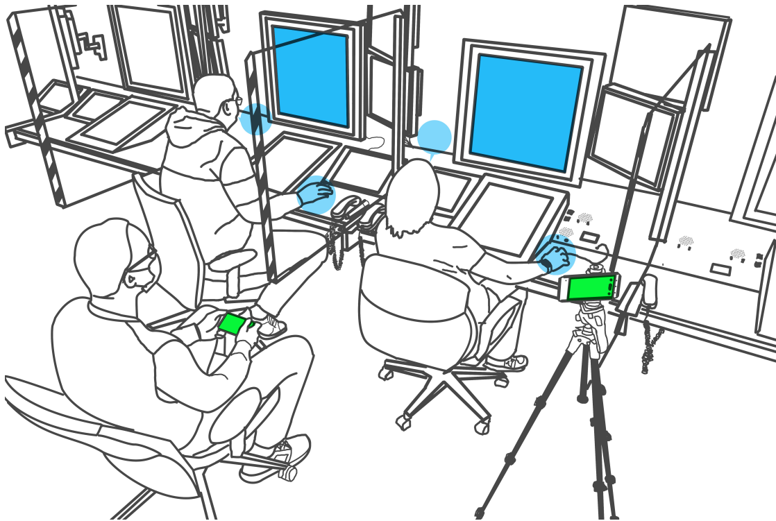
Figure 5.4: The sketch visualises the setup of the Proxemo deployment in the simulation. The approach controllers are sitting at their workstations on the positions pickup (left) and feeder (right). They use a mouse to document clearances and interact with traffic displayed on the large radar screen and communicate with each other directly via voice (blue highlights). The supervisor is sitting behind them and documents observed emotions in the Proxemo App whose logfile will later be synchronised with the video recording of the feeders' workstation (green highlights).
