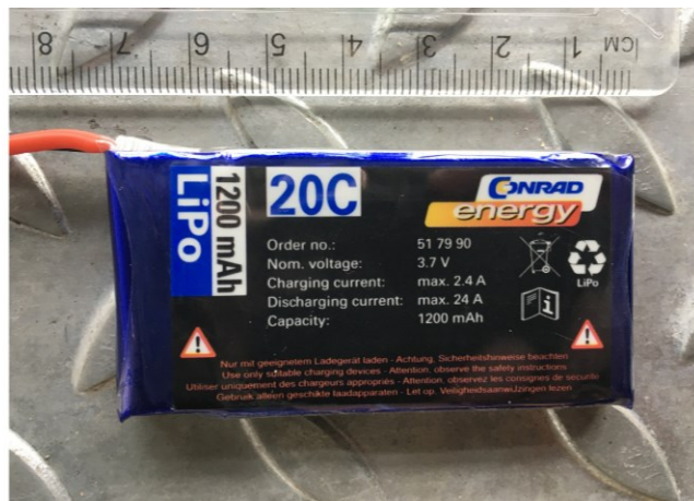
Figure 3.1: Studied cell as delivered by the supplier Conrad. The outer blue and dark polymer film can be removed to access the surface of the pouch foil directly.
