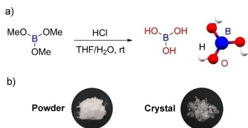
Figure 1. a) Synthesis of boric acid from B(OMe) 3 . b) Photographs of BA as a ground powder and as crystals, taken under daylight. The ground powder retains crystallinity.
