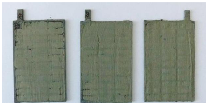
Figure 17: Manually pasted negative plates containing carbon additives after curing procedure.
