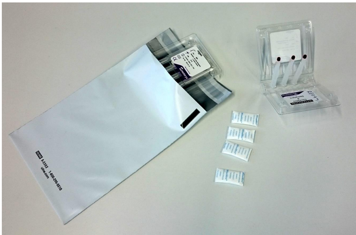
111 112 Figure 3. MITRA™ devices loaded with blood samples are boxed in a plastic casing for mechanical stability 113 and packed in a plastic bag (PP) including desiccant for shipment
