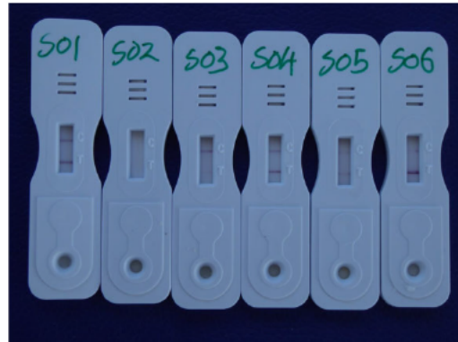
Figure 11: Positive (S01, S04, S06), negative (S03, S05) and invalid (S02) CCA-POCT tests.
