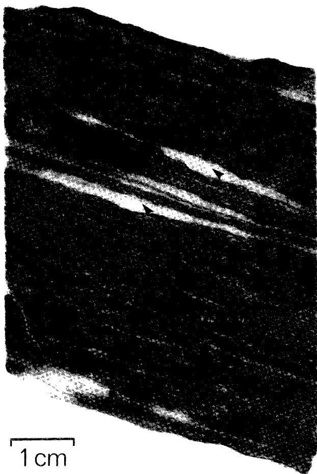
Fig. 2. Partly boudinaged (arrowheads) calc-silicate layers in gneisses which display porphyroblastic garnets (sample depth: 160 m).
