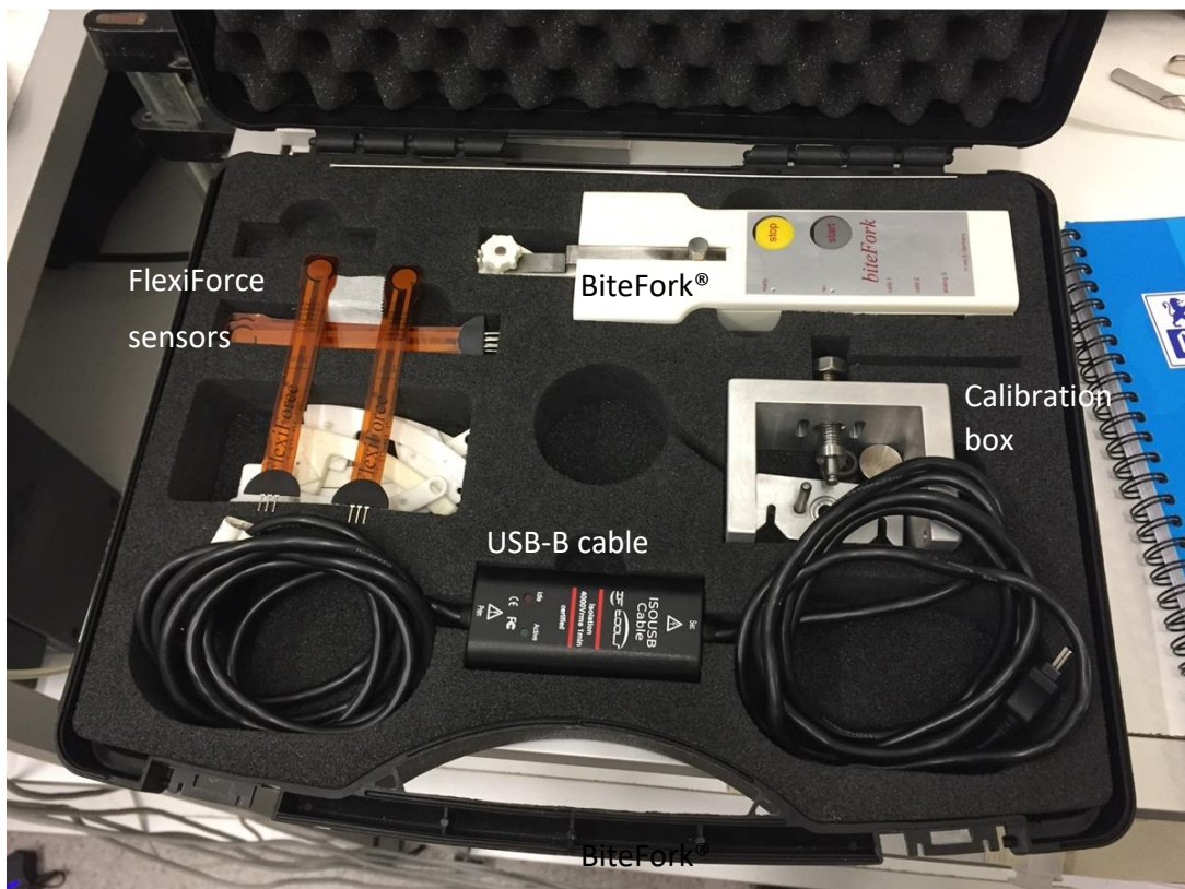
Figure 16: BiteFork® equipment, entailing the BiteFork® main device body, FlexiForce sensors, the USB-B cable, and the calibration device.
