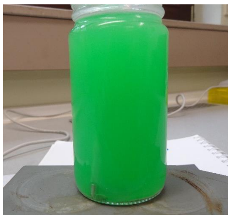
Image 4: Disintegration test of a Ghanaian ABZ sample.
