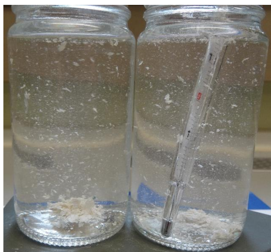
Image 12: Elyzole samples disintegrating too slowly and in thin flakes.
