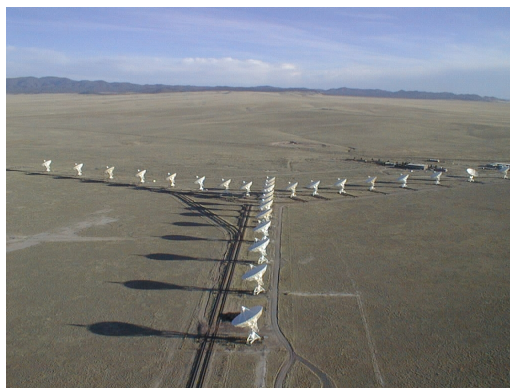
Figure 2.23: Aerial view of the VLA telescope in New Mexico (USA) in the most compact D-configuration. Credit: NRAO
