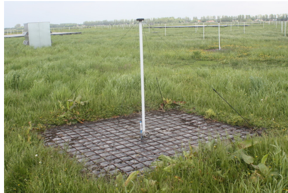
Figure 3.5: A single LBA element. The central PVC tube carries the cables to the top, where four dipoles are attached to the base edges at a 45° angle. There are 96 of these elements in a station. Credit: ASTRON/LOFAR
