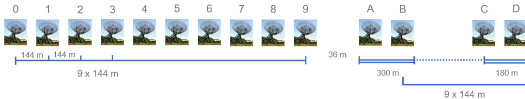
Figure 2.20: Schematic of the linear WSRT array. The first group of dishes (from left to right) are stationary, while dishes A, B, C and D are movable on tracks to create different baselines with desired properties.
