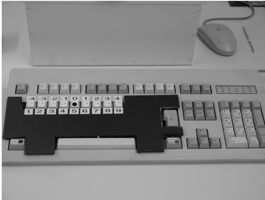
Figure 7: Close-up of the modified keyboard for rating input and experiment control.
