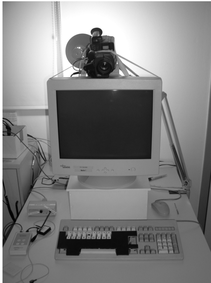
Figure 6: Experimental setup from the perspective of the participants. The picture shows the monitor for stimulus presentation with a video-camera on top for behavior observation in an adjacent room, the modified keyboard for rating input and experiment control, as well as the Varioport physiology data recorder on the left foreground of the table.
