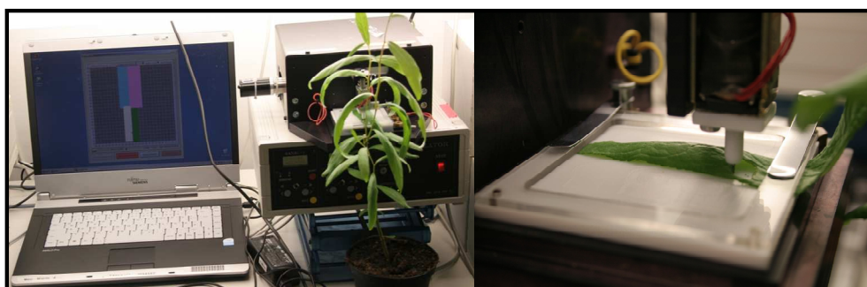
Fig.2.4 Mecworm, the mechanical caterpillar. Left, overview of the MecWorm system. Right, section of the punching unit of the Mecworm, including the aglet treating a P. trichocarpa leaf.
