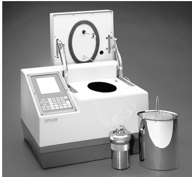
Abb. 4 Isoperiboles Bombenkalorimeter Parr 1266 (Fotoquelle: Parr Instrument)
