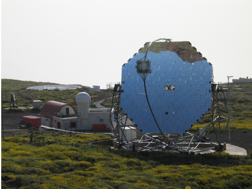
Figure 3.3: The MAGIC telescope on the Roque de los Muchachos in the Canary island of La Palma. It is currently the largest Cherenkov telescope worldwide.
