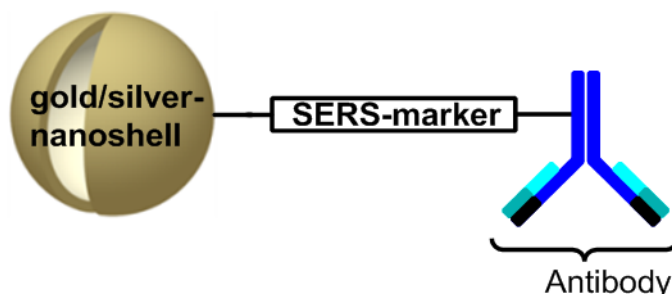
Scheme 19. Model of a biofunctionalized SERS-label. Left: Gold/Silver nanoshell. Middle: SERS-marker. Right: monoclonal antibody for antigen recognition (e.g. PSA).
