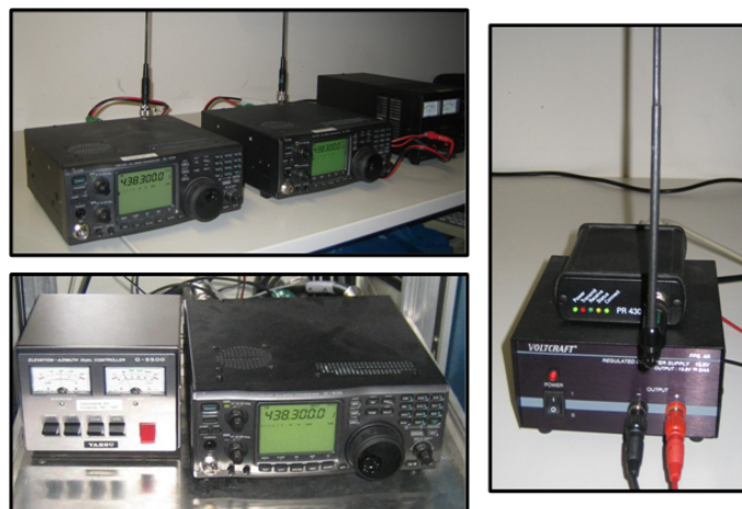
Figure 4.28: Hardware setup with 3 receiving stations using the ICOM 910 device. Transmitting station with PR430 transceiver
