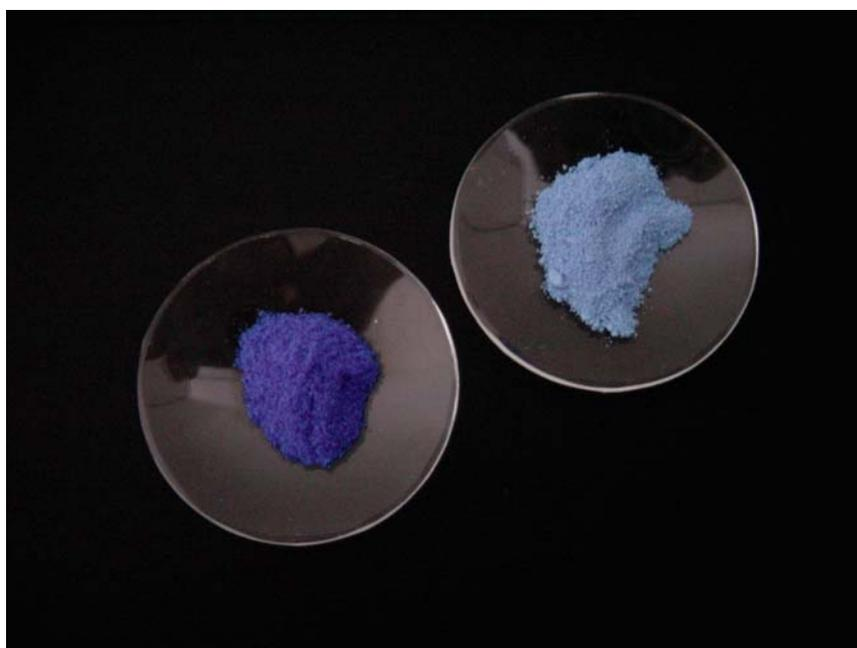
Fig. 5.3: Silica-nanoparticle with a value of TFPTMSi = 0.3 % (w/w), JA133-Si = 6.68  $\mu\text{mol/g}$  SiO<sub>2</sub>,  $\varnothing \approx 43$  nm (left); silica-nanoparticle with a value of TFPTMSi = 0.2 % (w/w), JA133-Si = 6.53  $\mu\text{mol/g}$  SiO<sub>2</sub>,  $\varnothing \approx 72$  nm (right).
