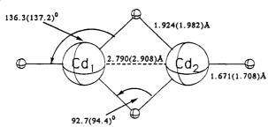
**Figure 1.** MP2(HF) optimized structure for Cd<sub>2</sub>H<sub>4</sub>: (a)  $C_{2h}$  minimum; (b)  $D_{2h}$  transition state.
