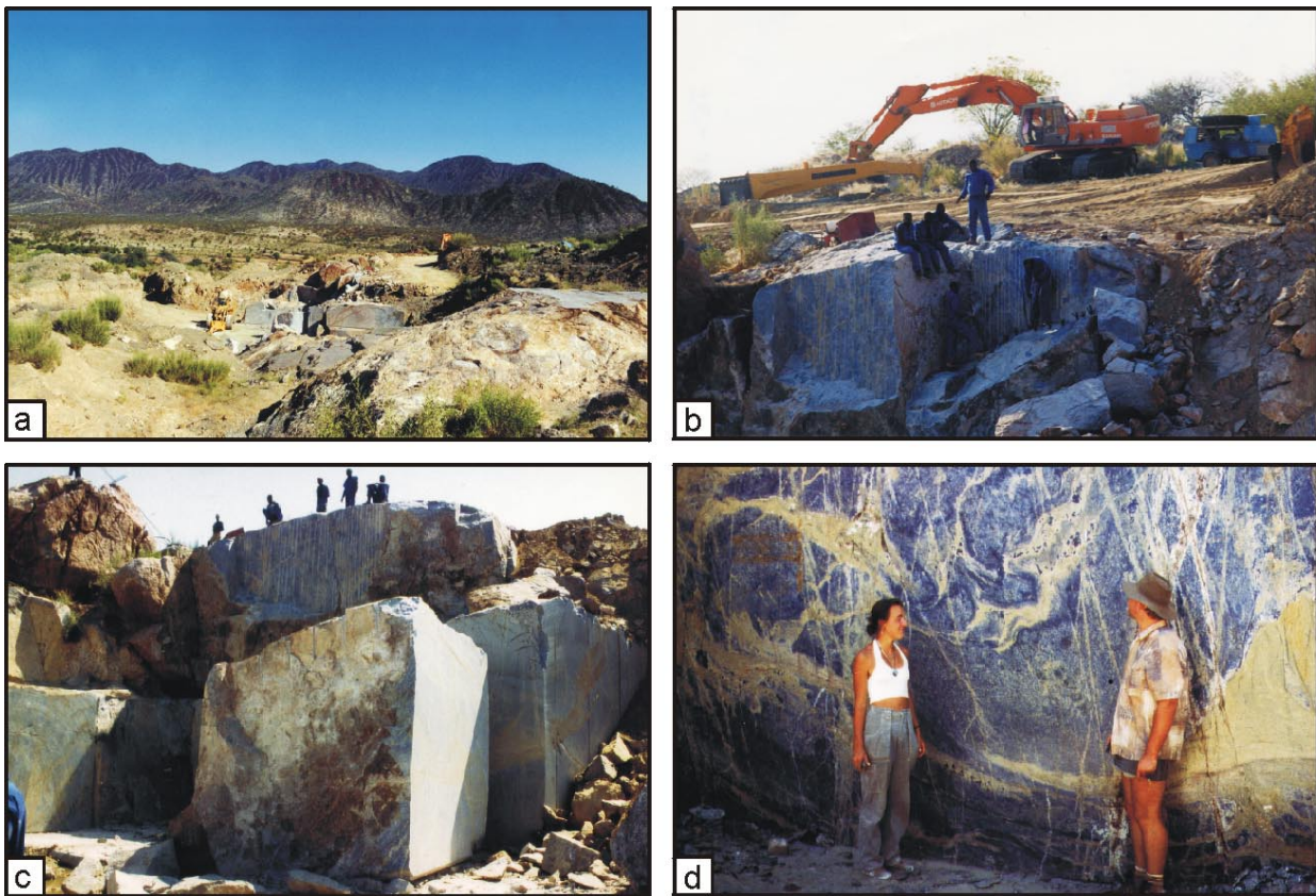
Fig. 3.9: Photographs of sodalite opencasting 8, which is the only opencasting that is presently mined (Locality: S 17°20.470', E 13°47.000'). a) The mine is situated in the central parts of a large carbonatite dyke, crosscutting leucogabbroites of the dark anorthosite suite. b) and c) Sodalite-rich lithologies are mined bench-like, with the sizes of the dimension stone blocks reaching up to 45 m 3 in a first step. d) Sodalite is enriched in the central parts of the carbonatite dyke. In these zones, sodalite (blue) replaces feldspar-rich xenoliths of up to 1.5 m in diameter, that are in turn surrounded by and intermingled with ankerite-rich zones (yellowish).
