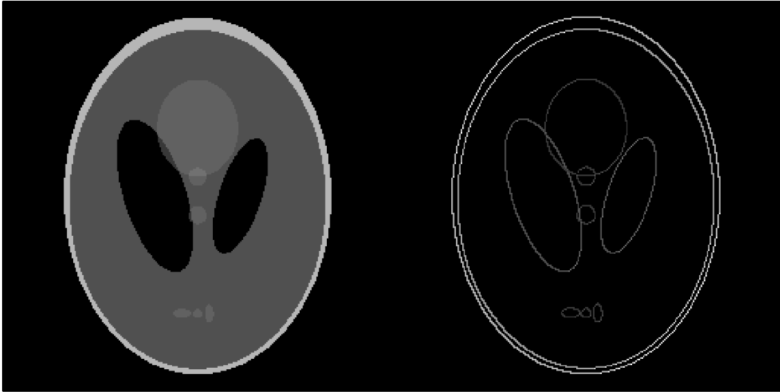
Figure 6: Left: The standard noise-free Shepp-Logan phantom that is not sparse in the image domain; right: The Shepp-Logan phantom after Discrete Gradient transform. Only the edges of the object are visible, leading to a very sparse description of the phantom.
