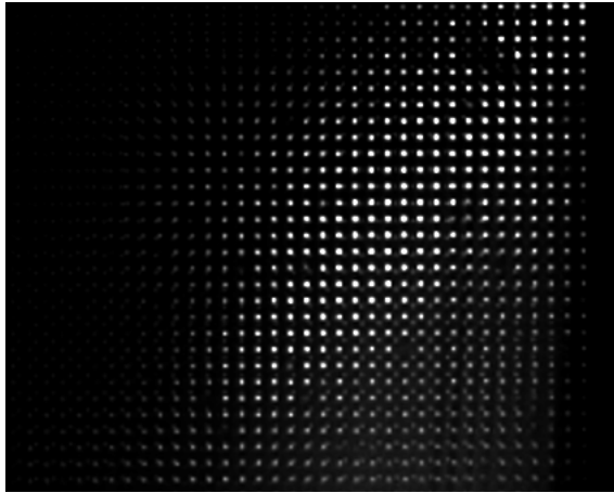
Figure 8.4: Example of a wavefront measurement with high-order harmonics. For some holes the transmission is reduced due to dust remaining inside the hole. From this image the wavefront and the beam profile of the high-order harmonics can be reconstructed.
