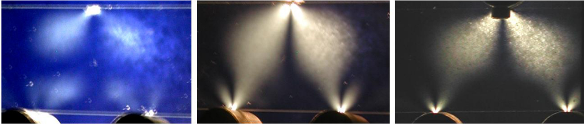
Fig. 46: Stress distribution in T5 targets: The situation of an unloaded pre-stressed sample (left) is depicted, as well as the stress distribution under the load of a 4,5 mm wide (center) and a round (right) hammer head.
