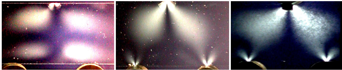
Fig. 50: Stress situation in T10 targets: An unloaded pre-stressed sample (left) is depicted as well as samples loaded by a pointed (center) and a round (right) hammer head.
