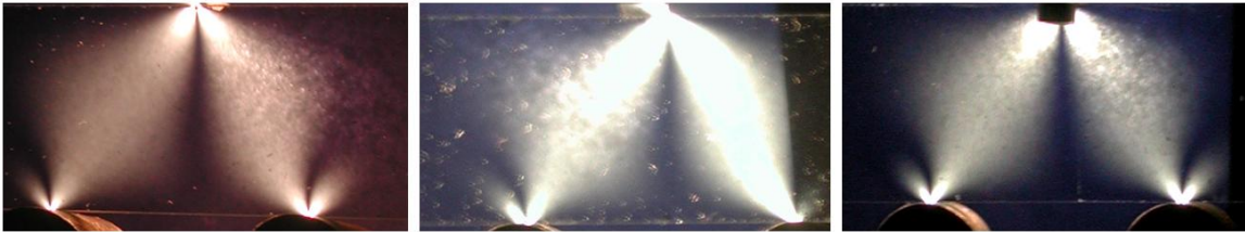
Fig. 43: Results of photoelastic investigations for FG: The stress distribution under static loading is depicted, using different hammer geometries (from left to right: {X11}; {X21} and {X31}).
