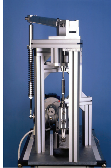
FIGURE 2: Test bench for cyclic load application on artificial ligament and fixation block.
