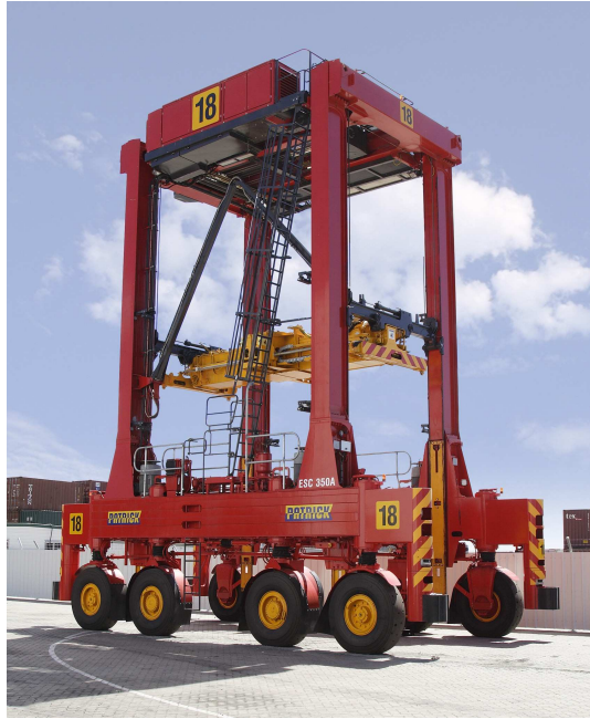
Figure 5.3: Automated straddle carrier AutoStrad from Kalmar Industries, Finland (photo courtesy of Kalmar Industries).
