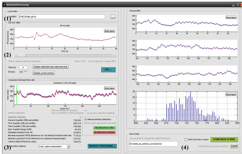
Fig. 3 The graphical user interface of the subprogram ibiArtifactProcessing. 1 Load data. 2 Raw data plot on a scrollable axis and the possibility to cut data manually. 3 Data plot with detected artifacts and
