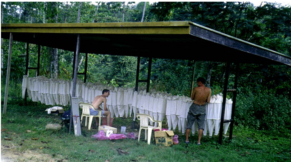
Fig. 11 120 mini Winkler sacks running in the shade for three days in Danum Valley.
