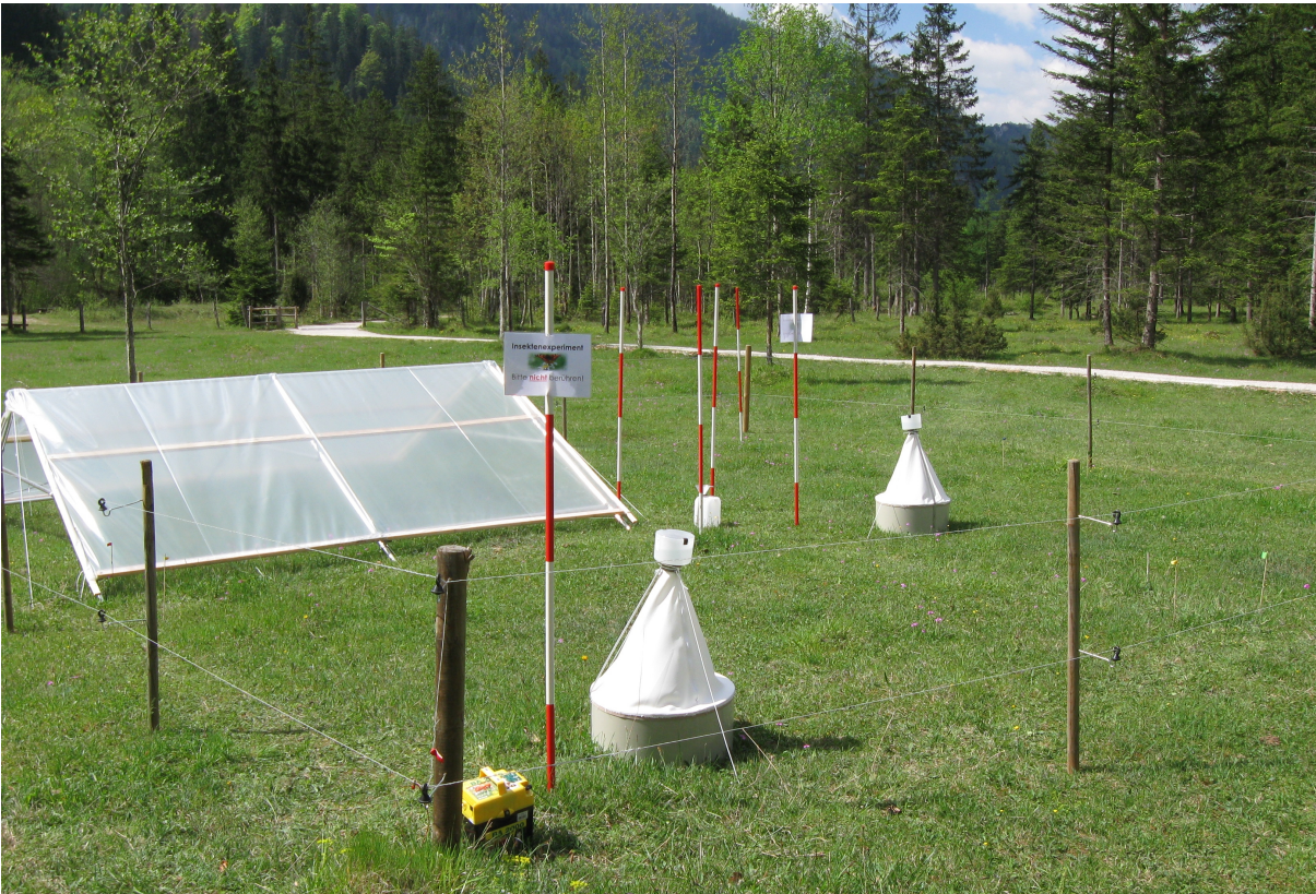
Fig. I.4: Fenced experimental site with a 4 x 4 m rain-out shelter to simulate an extreme drought event. Photo: B. Hoiß
