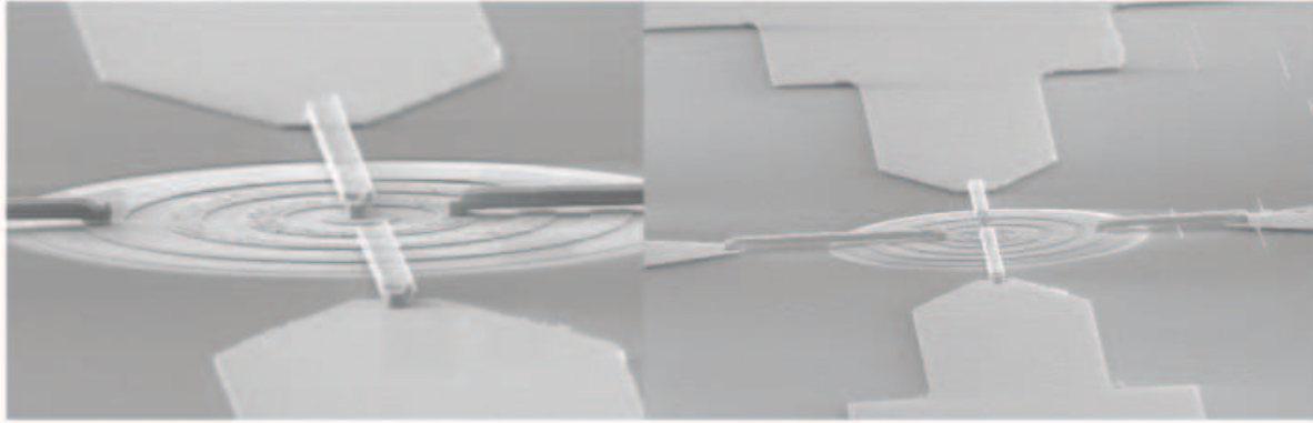
Fig. A.3: Typical errors encountered while making the device. On the right shows underexposed rings. The left-over resist form clumps on top of the rings, increasing the contact resistance dramatically. On the right shows leftover metal trapped between rings.
