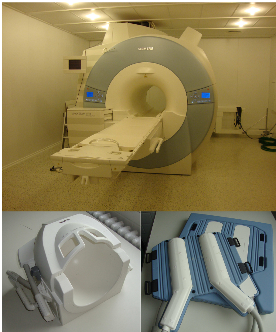
Figure 5.1: MRI System (top) and receiver coils (bottom) used in this thesis. 32-channel head coil (bottom-left) and 32-channel body coil (bottom-right) with its 16 anterior and posterior elements.
