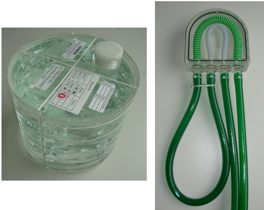
Figure 5.2: Stationary phantom (left) and flow phantom (right) used for in vitro studies.
