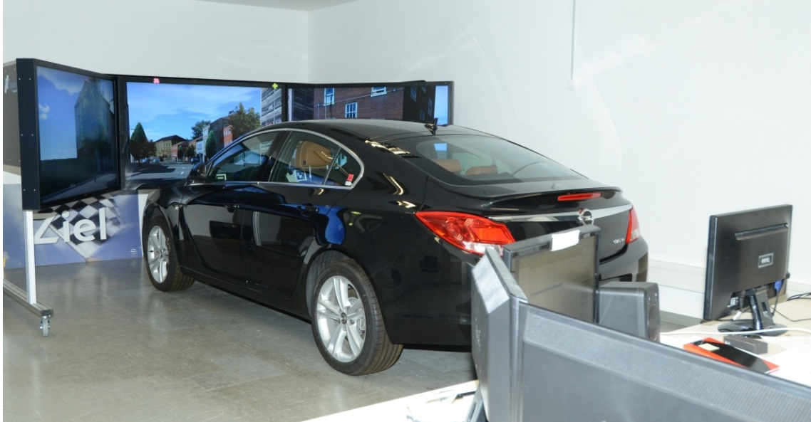
Figure 4.2: Simulator of the Adam Opel AG which was used for Study 2.
