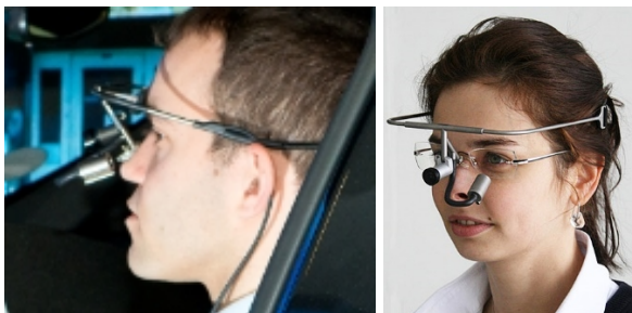
Figure 4.4: Dikablis eye-tracker which was used for Study 2.
